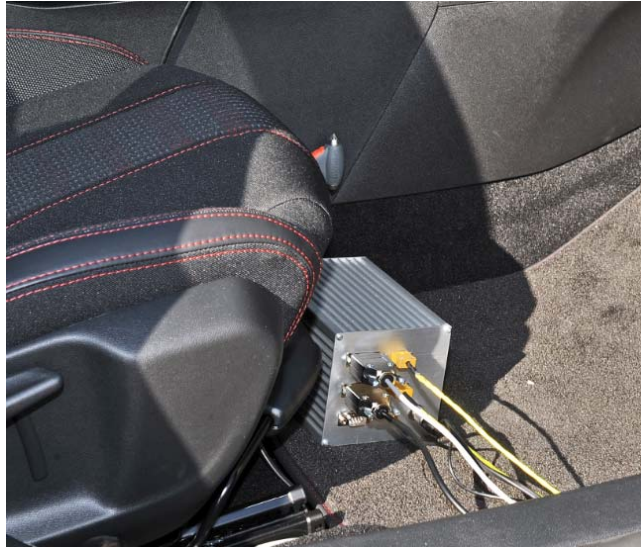
Figure 1.2: The SEMS datalogger with cabling to/from sensors, GPS, OBD and power connections.
