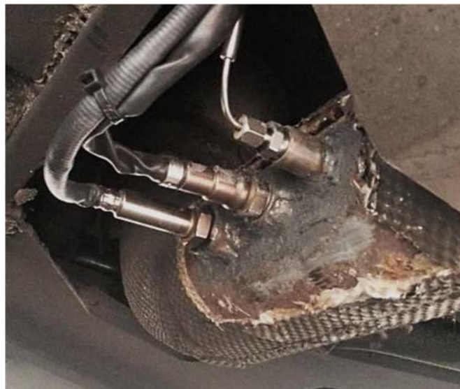
Figure 1.1: Example of sensors as used by SEMS, mounted in the exhaust of a vehicle.
