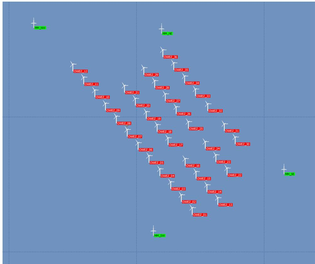
Figure 4-1 FarmFlow model of the OWEZ wind farm containing 36 wind turbines surrounded by four virtual met masts positioned on DOWA grid locations
