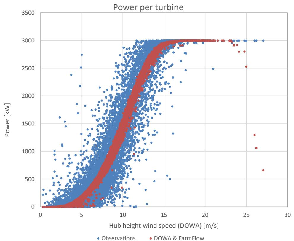
Figure 5-1 Comparison of the measured and simulated hourly power productions per turbine in OWEZ
