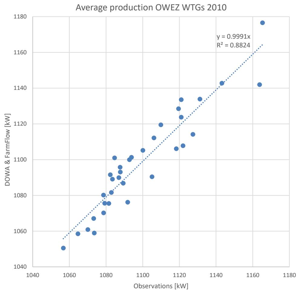
Figure 5-5 Correlation plot with linear least-squares regression of measured and simulated average productions of 34 OWEZ wind turbines in 2010
