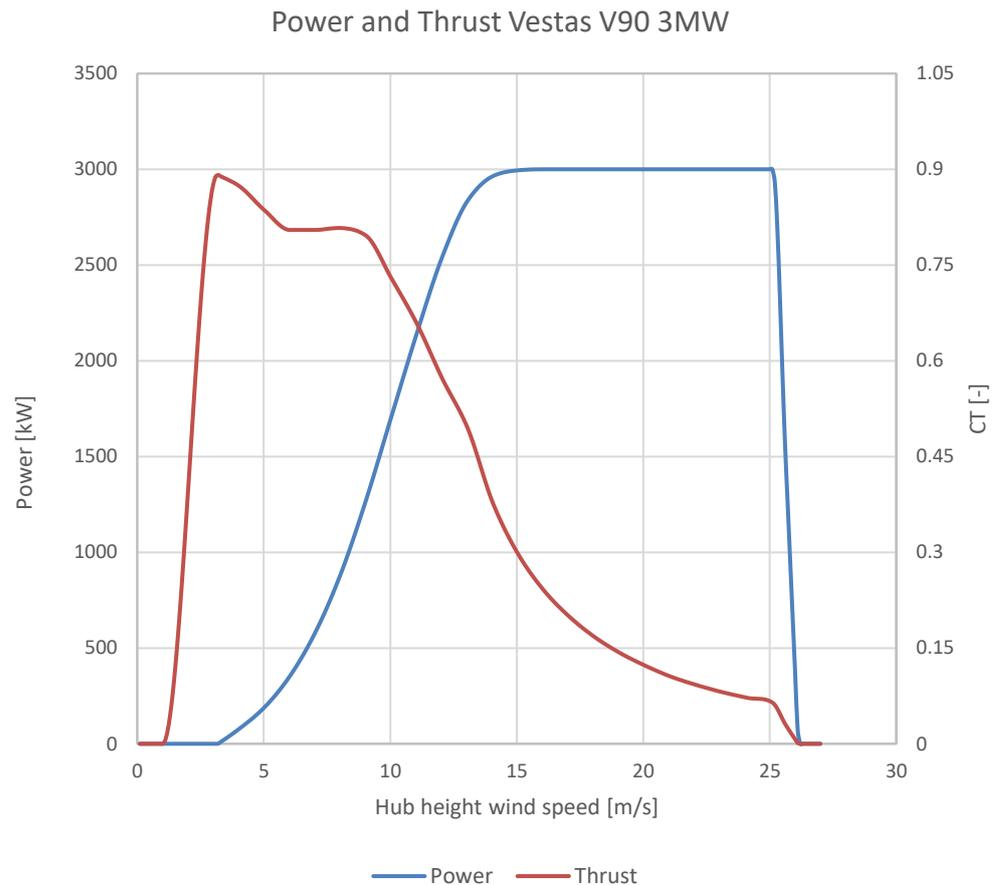
Figure 3-1 Standard power and thrust curve of the Vestas V90 3MW wind turbine
