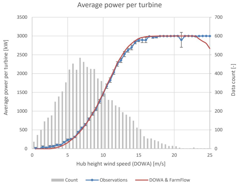
Figure 5-2 Comparison of the measured and simulated average power productions per turbine in OWEZ, including 95% confidence intervals (error bars) and a histogram of the used datapoints per wind speed bin
