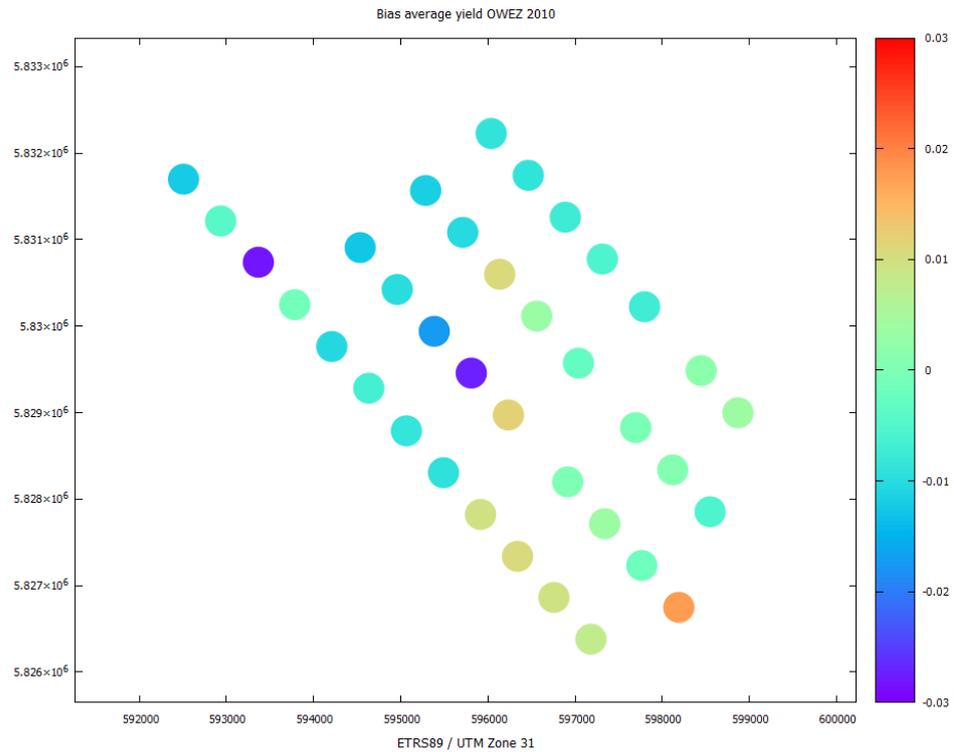
Figure 5-4 Bias of the simulated average yield of the OWEZ turbines in 2010 with DOWA wind
