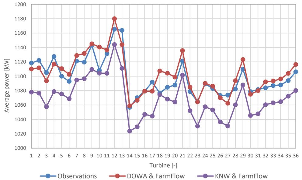
Figure 5-3 Comparison of the measured and simulated average power productions of individual turbines in OWEZ in 2010
