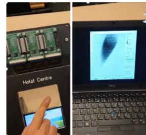
Transparent high-resolution photodetector: biometric-grade, collaboration with imec Leuven
