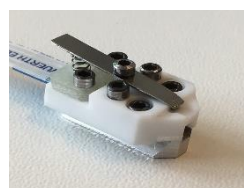
Realized design of Park AFM compatible tip holder with contact pins for electrostatically actuated membrane probes.
