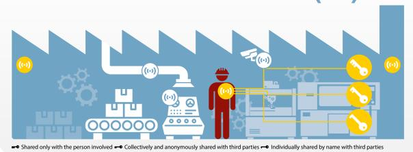
Stationary exposure sensors and modelling tools can be used to draw up concentration maps of workspaces. This can be done for more than one chemical substance simultaneously. If employees are fitted with an ILT device, individual exposure profiles can be developed by combining an individual's indoor location data with the concentration map data.
