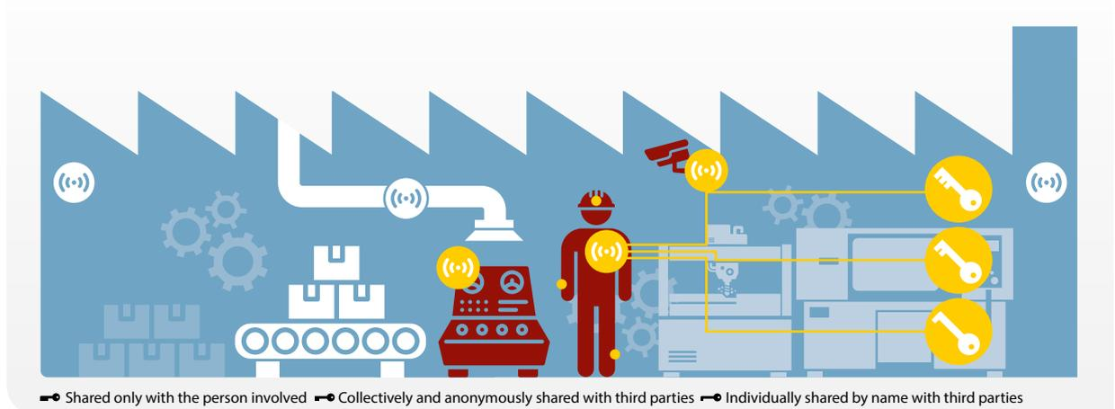
An exposure profile based on a personal exposure sensor is not easy to interpret. To understand what is causing peak or elevated exposures, insight is needed into what an employee has done, in what way, and under what circumstances, i.e. the context. This context can also be measured - in part - using sensors and other techniques, such as indoor location tracking, video cameras, and smart sensors that measure a person's posture or movement.
