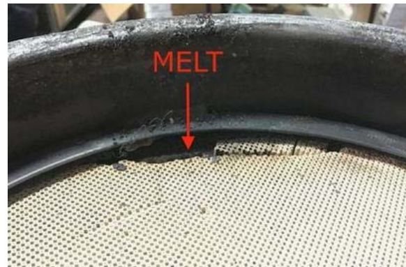
Figure 3.7: Example of molten filter, source Big Machine Parts
