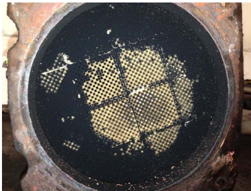
Figure 3.6: Example of clogged particulate filter, source Auto Expert
