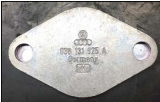
Figure 3.16: Genuine VAG EGR blanking plate for 1.9 and 2.0L 4-cyl diesel engine, source forums.vwvortex.com
