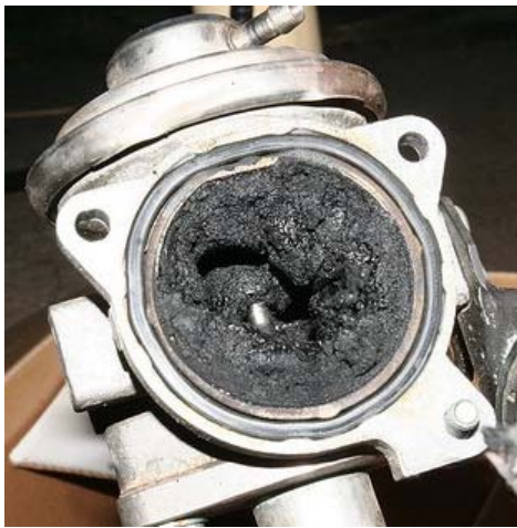
Figure 3.3: Example of a clogged EGR due to deposits, source Axle Addict
