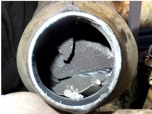
Figure 3.8: Example of cracked catalyst, source Viper Motorsports
