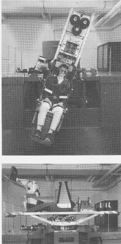
Figure 3.1. Two pictures showing the orientation of the TNO tilt chair for whole body roll about (a) an earth-horizontal axis and about (b) an earth-vertical axis. To illustrate the camera equipment for OT recordings, the hood was removed in (a). The roll axis was more or less centered between the eyes.
