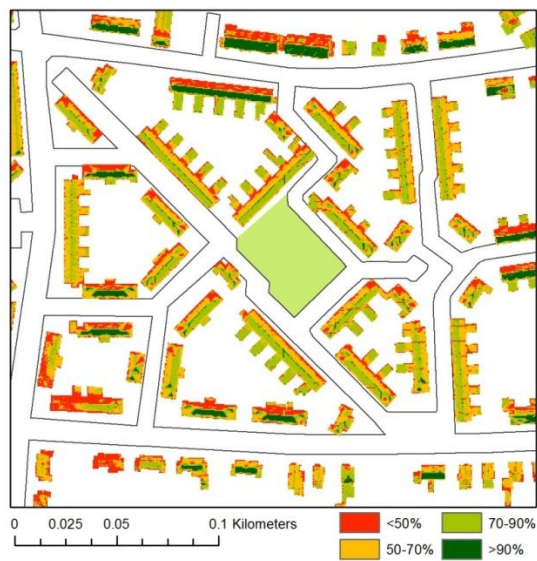
Figure 11: Final output of method 2 showing the PV rooftop potential in the city of Apeldoorn.
