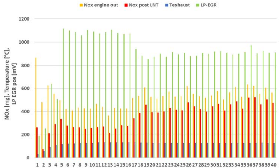
Figure 5-11: NO x emissions per ECE cycle with engine calibration 2 in a 10*UDC test with a cold start, start-stop active, performed on 07-05-2019. The test was started in a conditioning room of 25 °C and was conducted on the test track of the RDW at an ambient temperature of 13 °C. Preconditioning 3*EUDC with a warm start, conducted on 02-05-2018 with 3 LNT regenerations.
