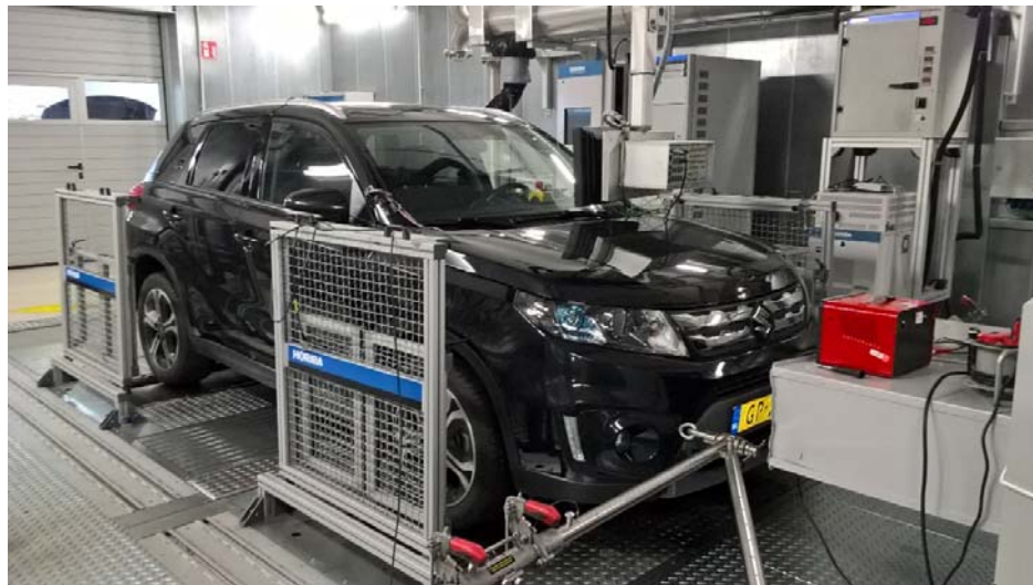
Figure 3-2: Chassis dynamometer and measurement equipment for performing an emissions test
