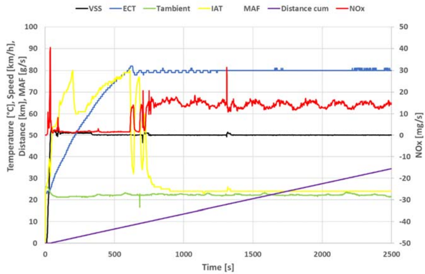
Figure 4-15: NO x emissions during a cold start with engine calibration C1 and a constant speed of 50 km/h. During the period in which the coolant temperature is rising (ECT is 20 - 80 °C), the NO x emissions are less than 2 mg/s. The NO x emission of the warmed up engine (ECT is 80 °C) is 11 – 17 mg/s.
