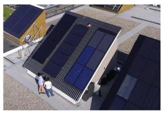
Fig. 2: Field test with three types of uncovered PVT systems on the dummy roof
