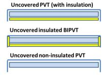
**Figure 1:** Three different PVT concepts (bright blue line: PV module, blue block: thermal absorber with fluid channels, yellow: insulation)
