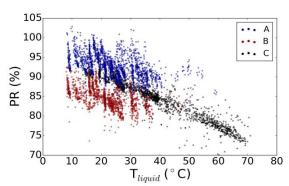
**Figure 5:** Correlation between the DC performance ratio and the average fluid temperature.
