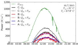
**Figure 3a:** Thermal (continuous lines,  $\dot{Q}_{th}$ ) and additional electrical power output (dashed lines,  $\dot{Q}_{th}$ +P<sub>PV</sub>) per m<sup>2</sup> for a day with a fluid input temperature of 35°C. In-plane irradiance ( $G_{POA}$ ) is shown in green.
