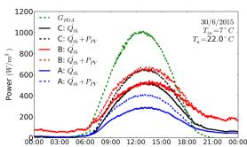
**Figure 3b:** Thermal (continuous lines,  $\dot{Q}_{th}$ ) and additional electrical power output (dashed lines,  $\dot{Q}_{th}+P_{PV}$ ) per m<sup>2</sup> for a day with a fluid input temperature of 7°C. In-plane irradiance ( $G_{POA}$ ) is shown in green.
