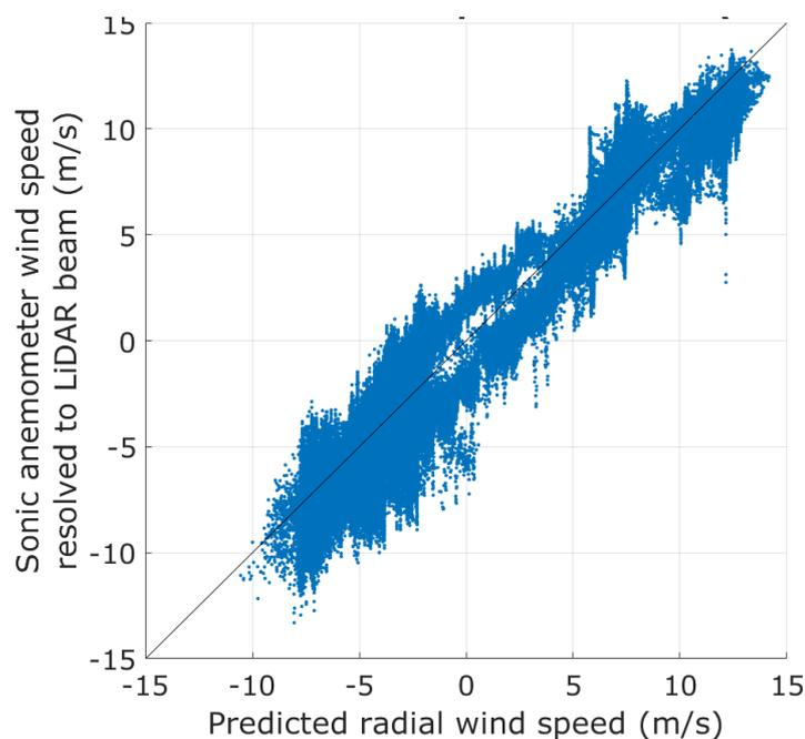
Figure 10 Scatter plot of sonic anemometer measurements, resampled at 1Hz and resolved to the LiDAR beam angle, versus predictions from the Virtual Lidar.
