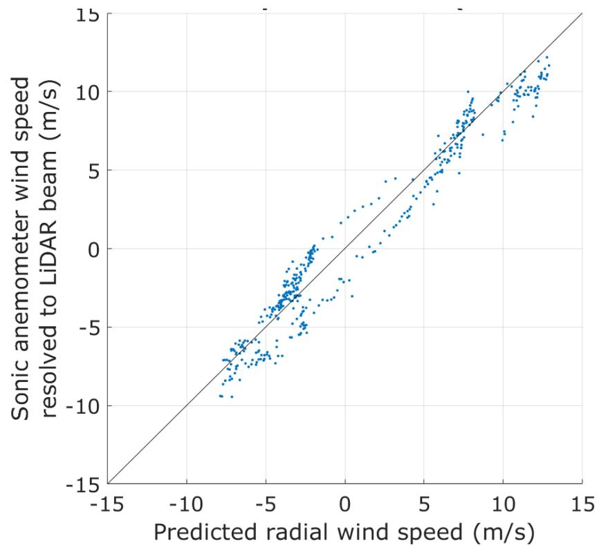
Figure 11 Scatter plot of sonic anemometer measurements, resolved to the LiDAR beam angle, versus predictions from the Virtual Lidar; both averaged to 10 minutes.
