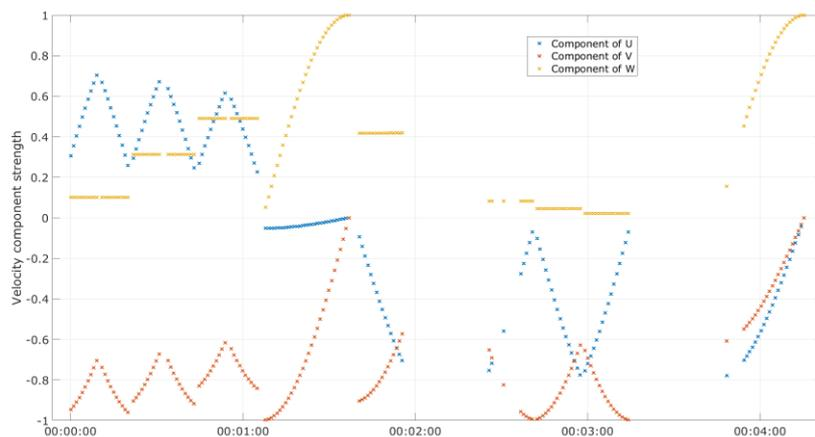
Figure 7 Example data from one iteration of all scanning patterns in time, showing the information content available for each component of the wind velocity (U: north, V: east, W: vertical)
