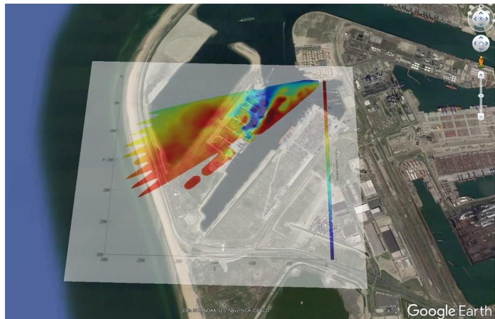
Figure 12 Radial wind speed at 50m height on 3rd of October, 18:20:22. The wind direction measured by the meteorological mast wind vane at this time is 205° (SSW).
