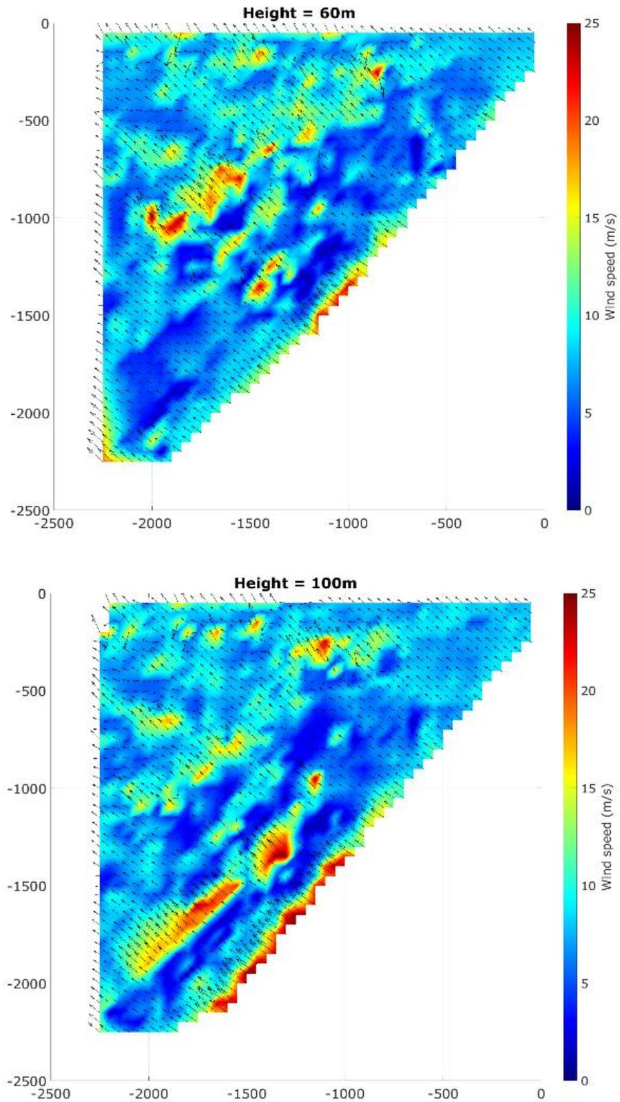
Figure 15 10-minute averaged wind fields, output at three heights (top to bottom: 20m, 60m, 100m) for 5<sup>th</sup> October 2019 20:30–20:40. The colours and arrows indicate the horizontal wind speed and direction.
