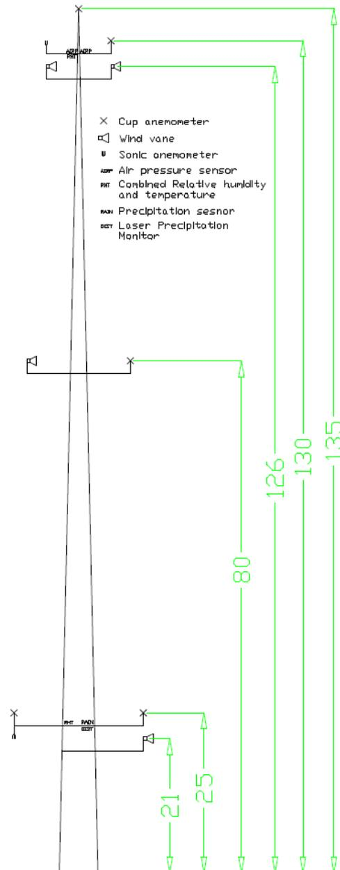
Figure 4 Meteorological mast heights and sensor layout
