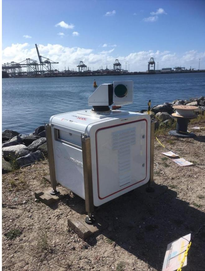
Figure 3 Windcube WLS-200S at the SIF site
