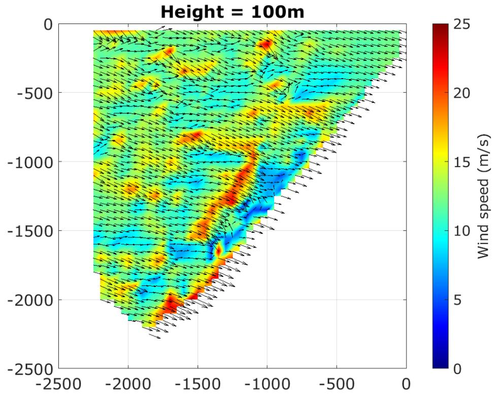
Figure 14 10-minute averaged wind fields, output at three heights (top to bottom: 20m, 60m, 100m) for 4<sup>th</sup> October 2019 14:30–14:40. The colours and arrows indicate the horizontal wind speed and direction
