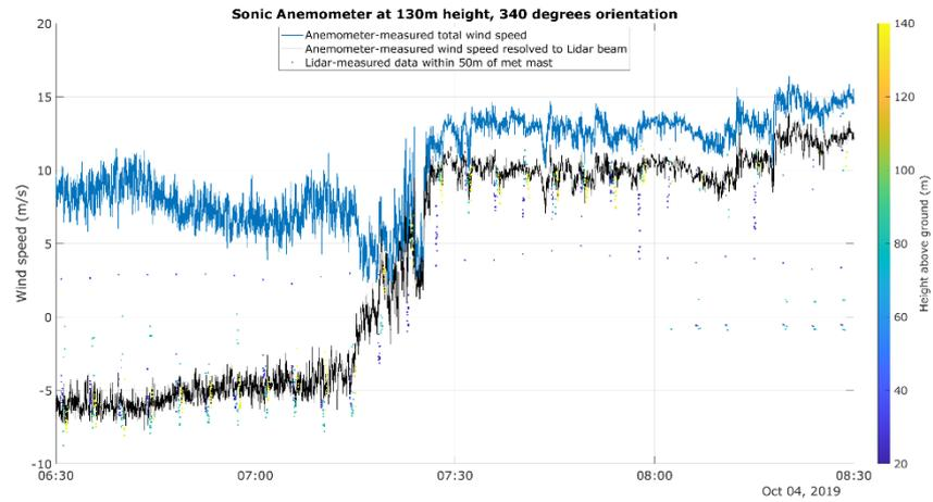
Figure 8 A two hour period during the campaign, showing the sonic anemometer-measured total wind speed (blue line), the wind velocity resolved to the LiDAR beam direction (black), and scanning LiDAR measurements (coloured dots) within a 50m zone around the meteorological mast. The colours of the LiDAR measurement points indicate height.
