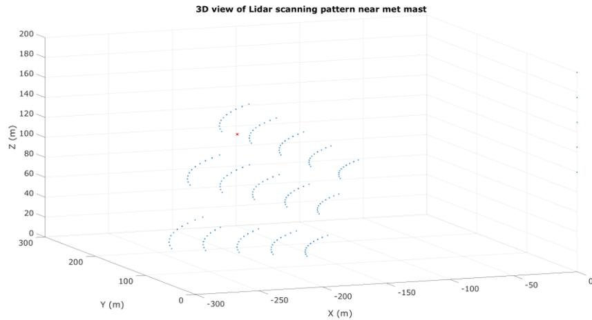
Figure 6 3D plot of example data from one iteration of the scan pattern in the northwest direction, with the sonic anemometer marked as a red cross.
