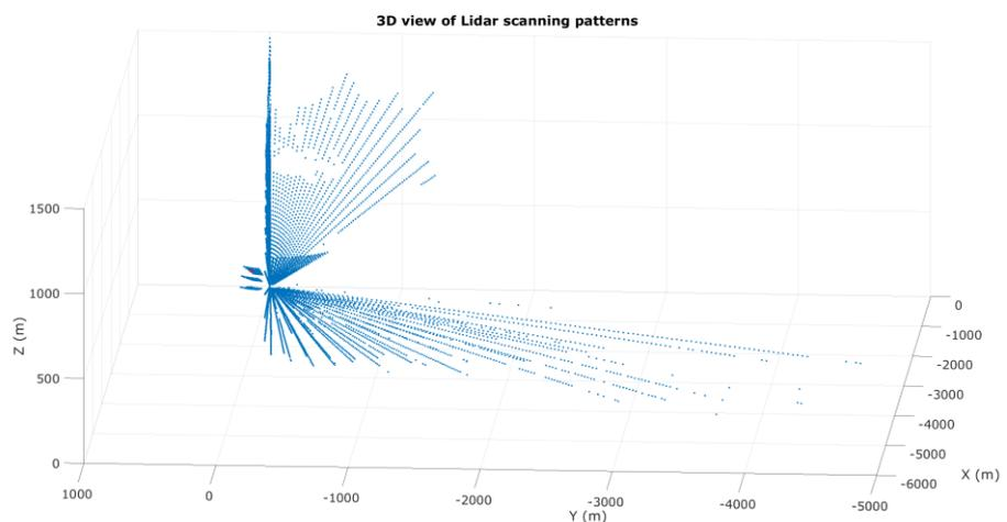
Figure 5 3D plot of example data from one iteration of all scanning patterns. Positive Y direction indicates North and positive X direction indicates East.
