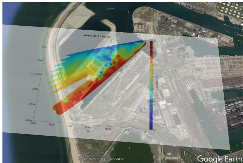
Figure 13 Radial wind speed at 50m height on 3rd of October, 23:32:33. The wind direction measured by the meteorological mast wind vane at this time is  $161^\circ$  (SSE).
