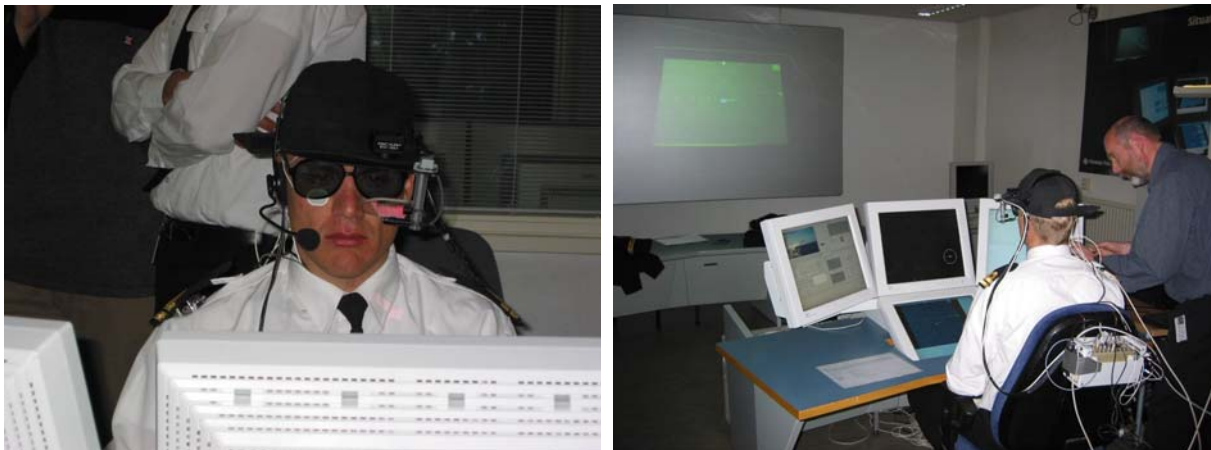
Figure 7: Pictures of an Air Defence Officer during the Tests, Equipped with Mini-Cameras, Sensors and Electrodes. Polarization glasses are used to see the stereo images.
