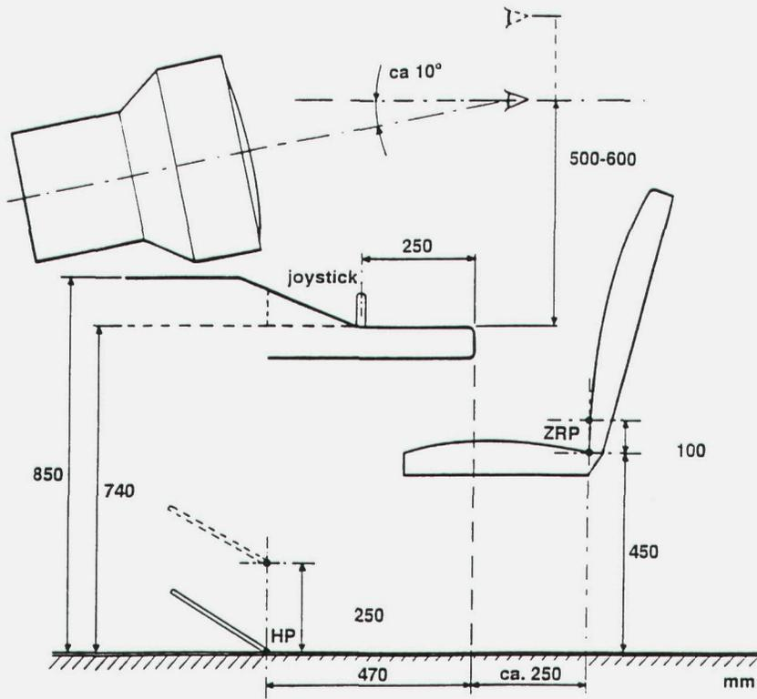
Fig. 7 Schematic side view of the TNO RPV research facility.
