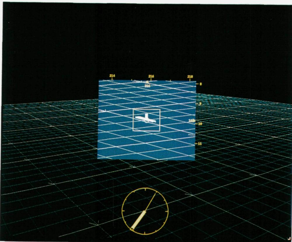
Fig. 2 The Computer Generated Grid (CGG), the camera image, and the Combined Heading and Pitch Indicator (CHPI) used in the current experiment.
