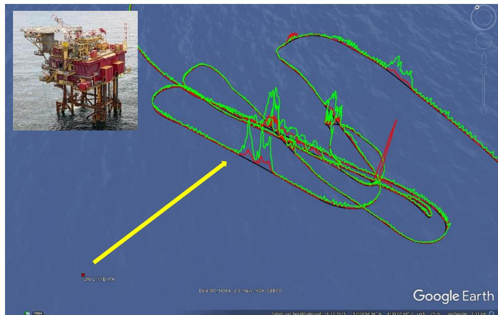
Figure 22 L11 measurements plotted in Google Earth, red= $\text{CH}_4$ , green= $\text{C}_2\text{H}_6$ .
