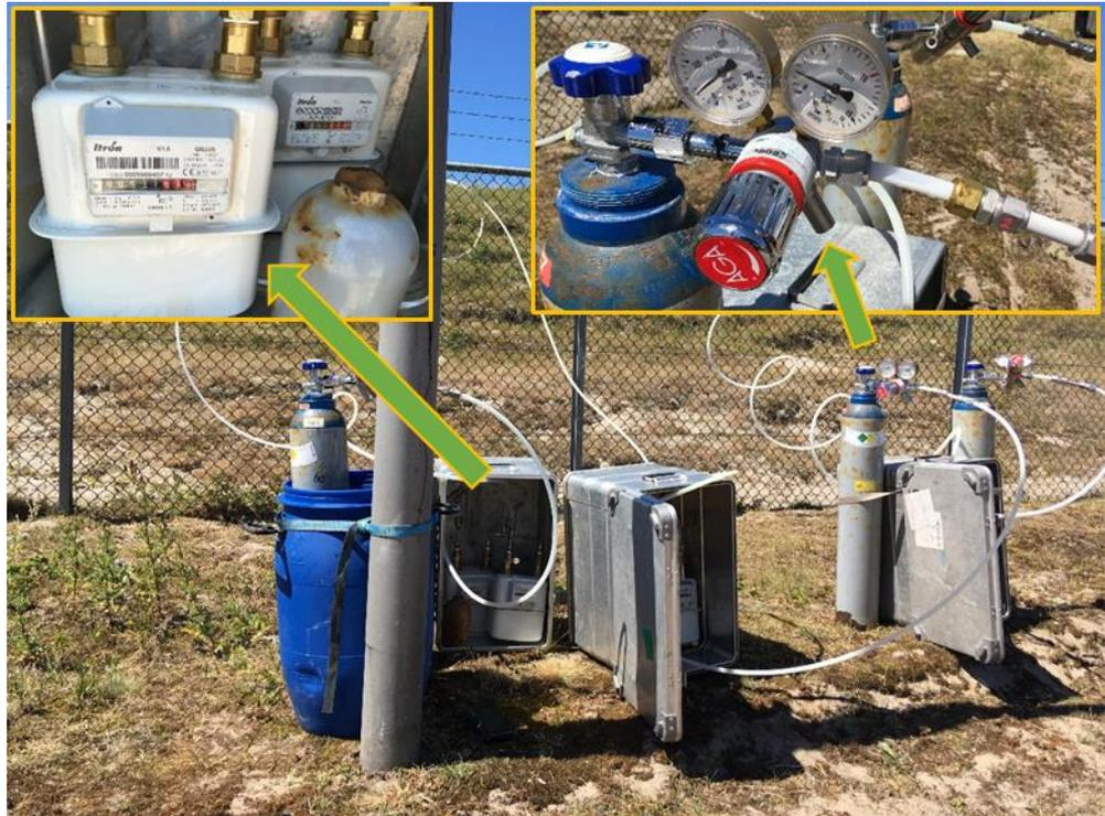
Figure 17 Example of the N<sub>2</sub>O release; left insert shows the flowmeters; right insert shows the pressure regulator and critical capillary.
