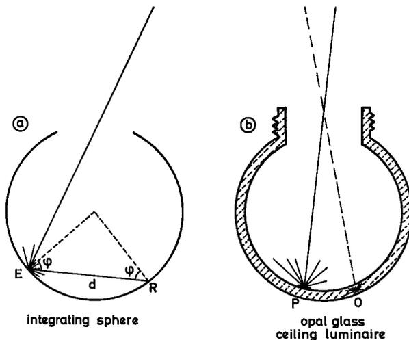
Fig. 7. a. In an integrating sphere, an increase in mutual distance  $d$  is compensated in its effect by a decrease in  $\varphi$ , so that the sphere is uniformly bright all over its surface.
