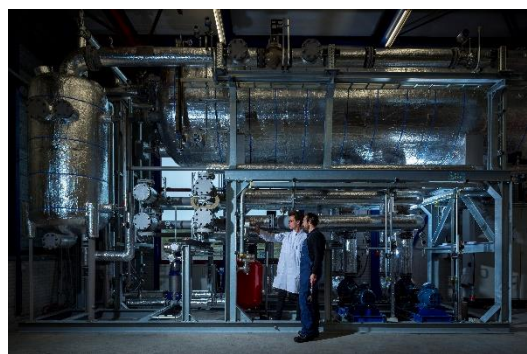
2MW heat pump test facility as part of the Carnot lab
