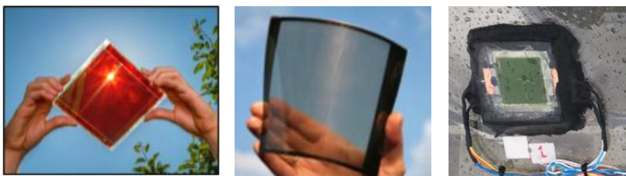
Examples of semi-transparent and see-through thin-film PV products, and a PV tandem module after a field test (very limited degradation).
