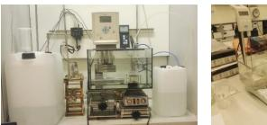
Development of cementitious binders based on secondary materials: Custom-built flow though experimental set-up to determine the dissolution rate of the binder precursors and effects of the activators on dissolution (left) and adapted reverse osmosis experimental set-up to determine the precipitation point (and solution-/precipitationproducts) (right).
