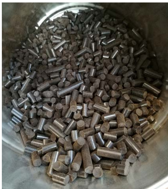
Figure 1 First batch of TORWASH® sewage sludge pellets
