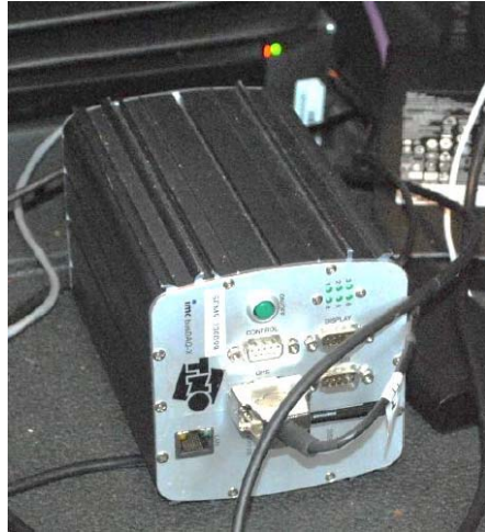
Figure 5: Smart Emissions Measurement System. SEMS was installed to measure boil-off frequency during normal operation at the Transport Company. Results yet to be published.
