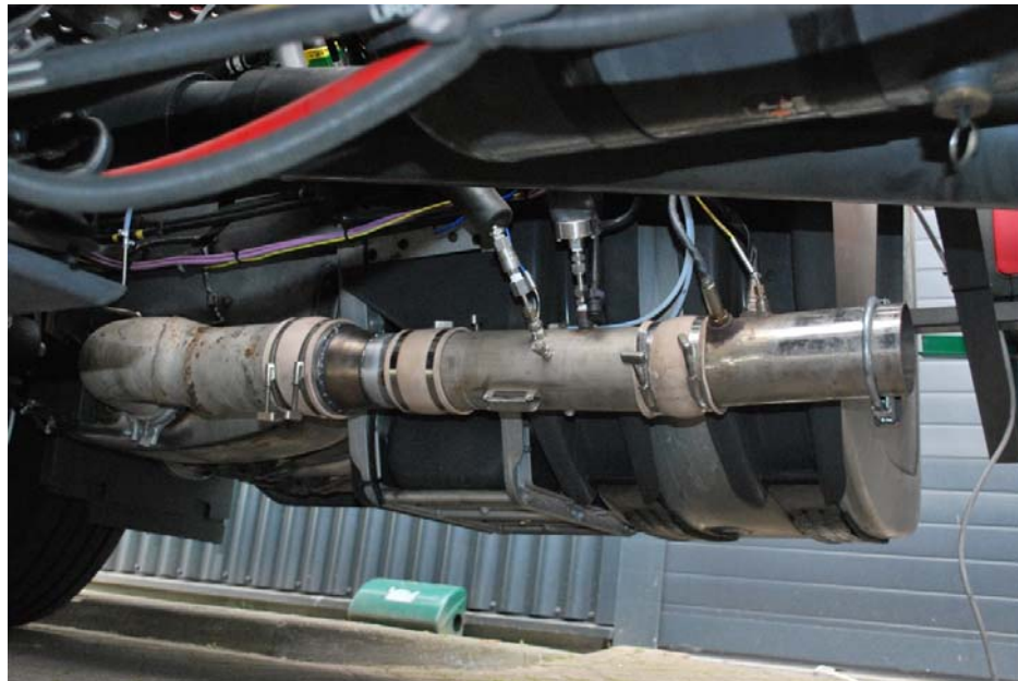
Figure 4: The flow tube connected to the exhaust of the truck.
