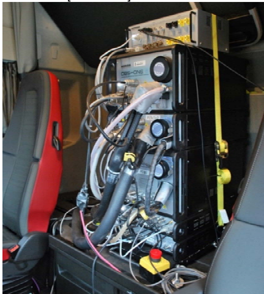
Figure 3: The PEMS analyser mounted in the cabin of the truck.
