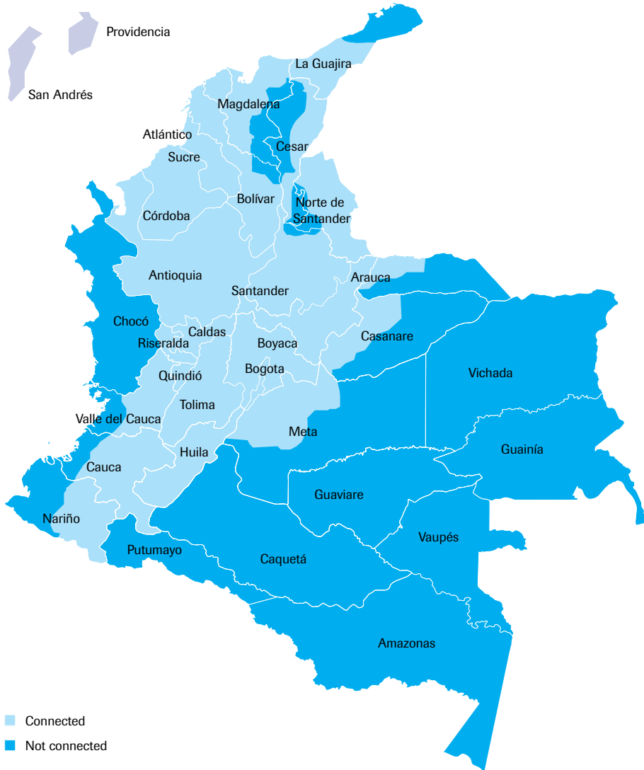
Figure 5 Coverage of National Interconnected System (NIS)
