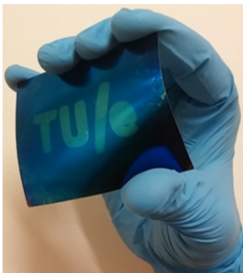
Figure 6. Pattern prepared by direct-write ALD of a 35 nm thick \text{In}_2\text{O}_3:\text{H} film on a flexible stainless steel foil covered with 20 nm of a-Si:H. This serves as a first demonstrator of the capability of the direct-write ALD process for large-area and flexible electronics.
