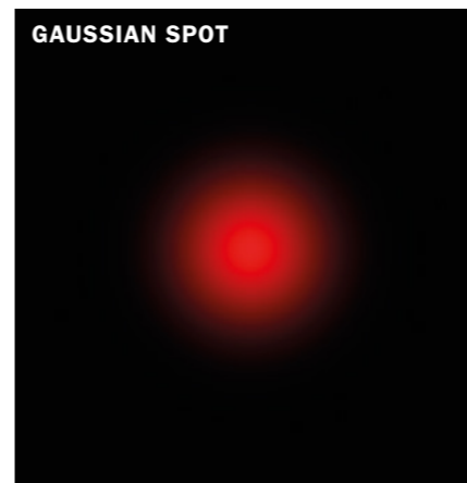
The combination of a diffraction limited Gaussian spot and a donut beam, resulting in an effective illumination spot that is significantly smaller than the diffraction limit of the optical system.
