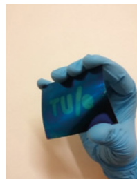
Figure 1. Logo created by direct-write ALD of 35 nm thick In 2 O 3 :H on flexible steel foil covered with 20 nm a-Si:H.
