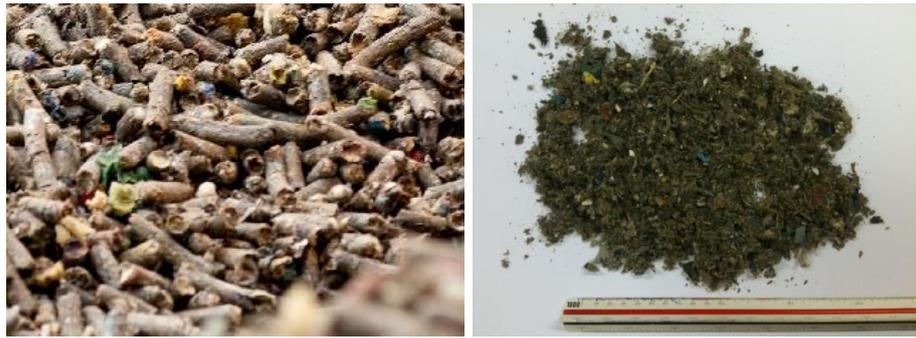
Figure 5 ICOPOWER® energy pellets, before and after shredding.
