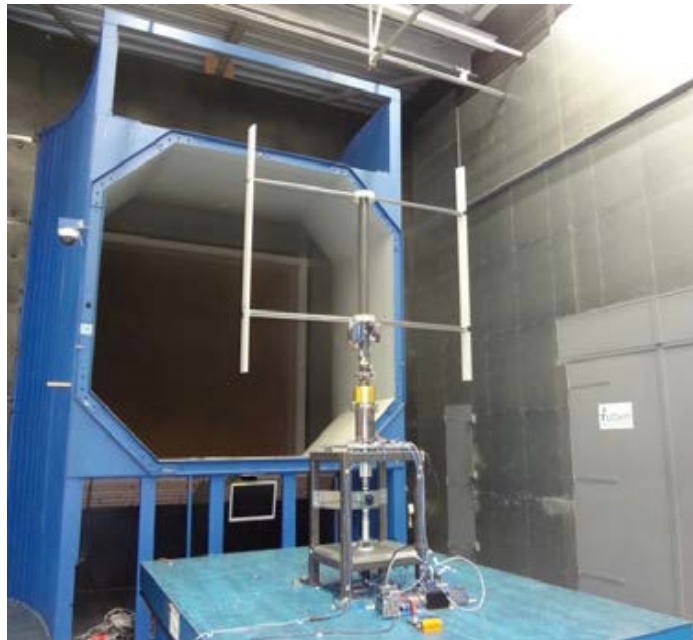
Figure 2.3: The scaled model for the wind tunnel measurement campaign
