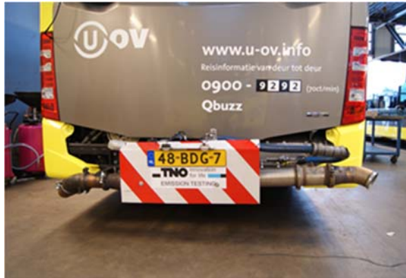
Figure 3: PEMS exhaust flow meter installed on the exhaust of the Mercedes Citaro.
