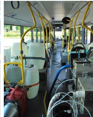
Figure 4: PEMS analyzers, additional equipment and payload inside the bus.
