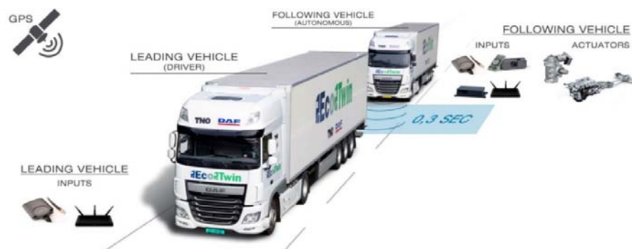
Figure 7: Truck platooning: trucks driving in convoy formation at short inter-vehicle distances using radar, cameras, GPS, and wireless connection
