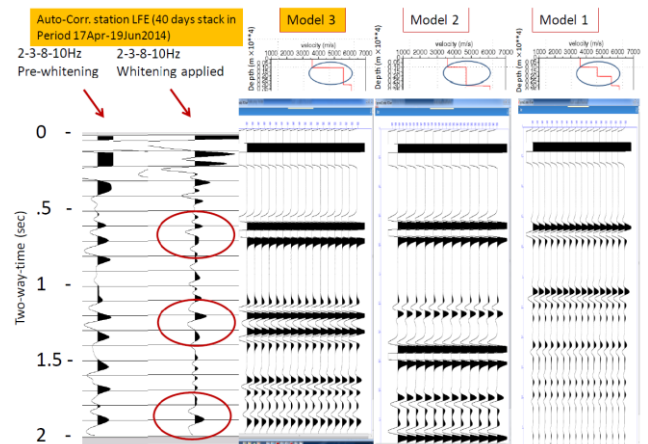
Figure 5: ANSI-processed autocorrelation stack for station LFE (two traces on left) and modelled global reflections for three velocity scenarios (modelled traces are repeated for convenience). Notice the encouraging match between the whitened field data result and the result computed for Model 3.
