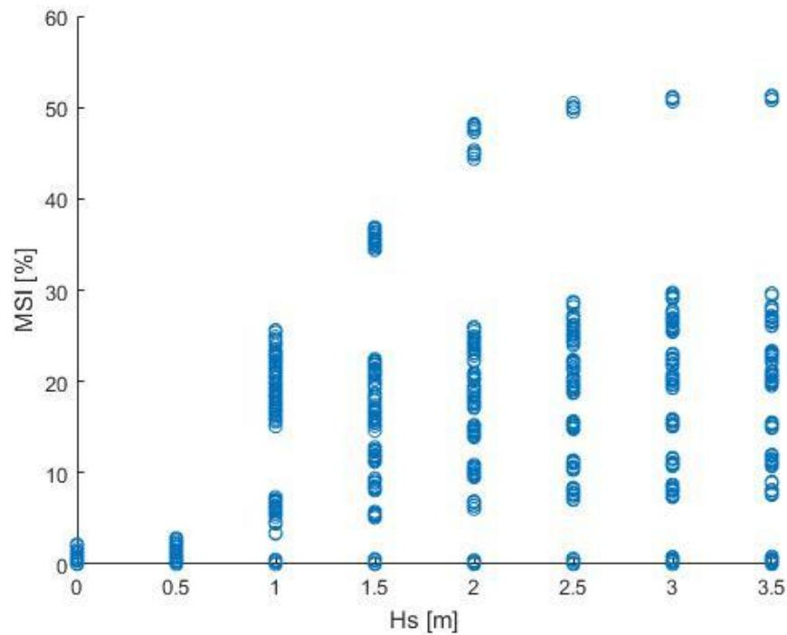
Figure 10 Motion sickness incidence versus significant wave height for 20-metre Catamaran (CTV)
