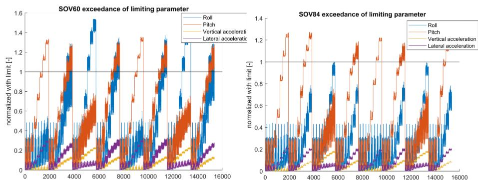
Figure 8 Exceedance of limit for all entries in the hydrodynamic database (limit given in root mean square, response parameter as standard deviation)
