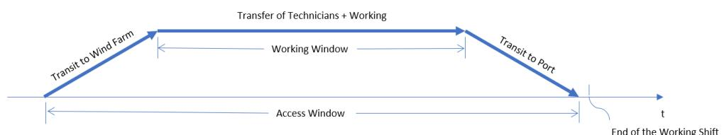
Figure 2 Illustration of the old approach used to determine an access window
