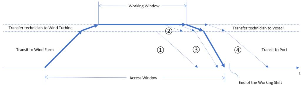
Figure 3 Illustration of the new approach used to determine an access window. The dotted lines represent options that are not selected.
