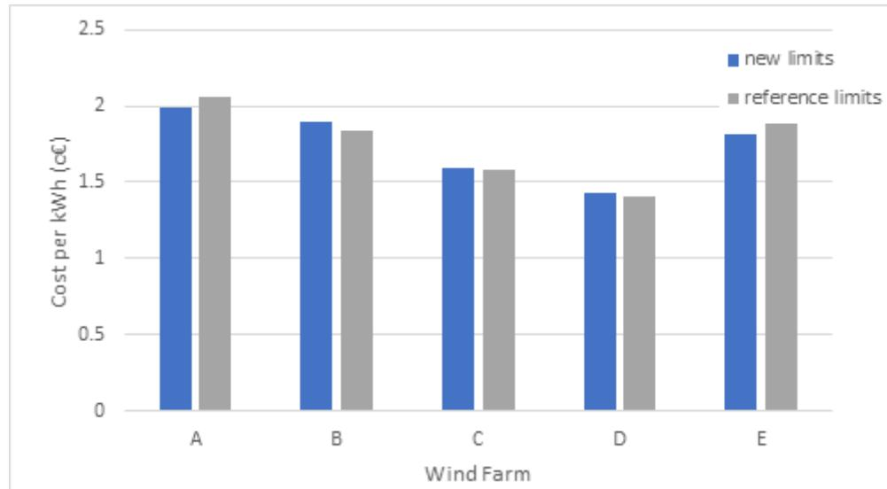
Figure 16 Comparison of cost per kWh for all wind farms in reference and new limits scenario
