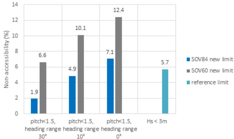
Figure 9 Sensitivity of non-accessibility for different heading ranges, compared to typical limit in reference study ( $H_s < 3m$ )
