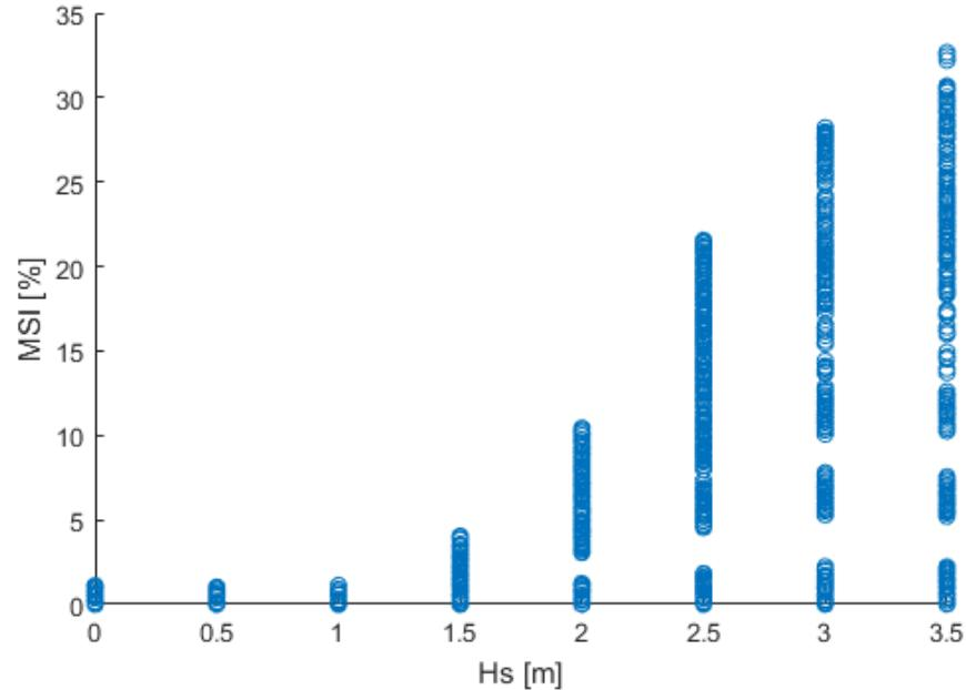
Figure 11 Motion sickness incidence versus significant wave height for 60-metre SOV
