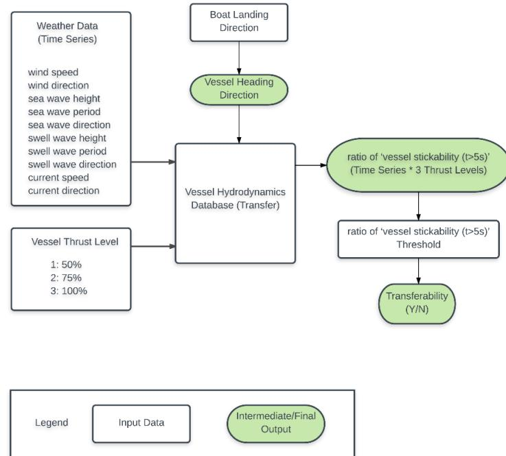
Figure 5 Illustration of the new approach to assess the CTV vessel transferability
