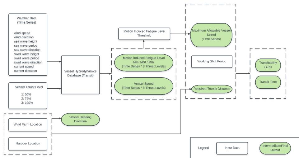
Figure 4 Illustration of the new approach to assess the vessel transitivity and transit time
