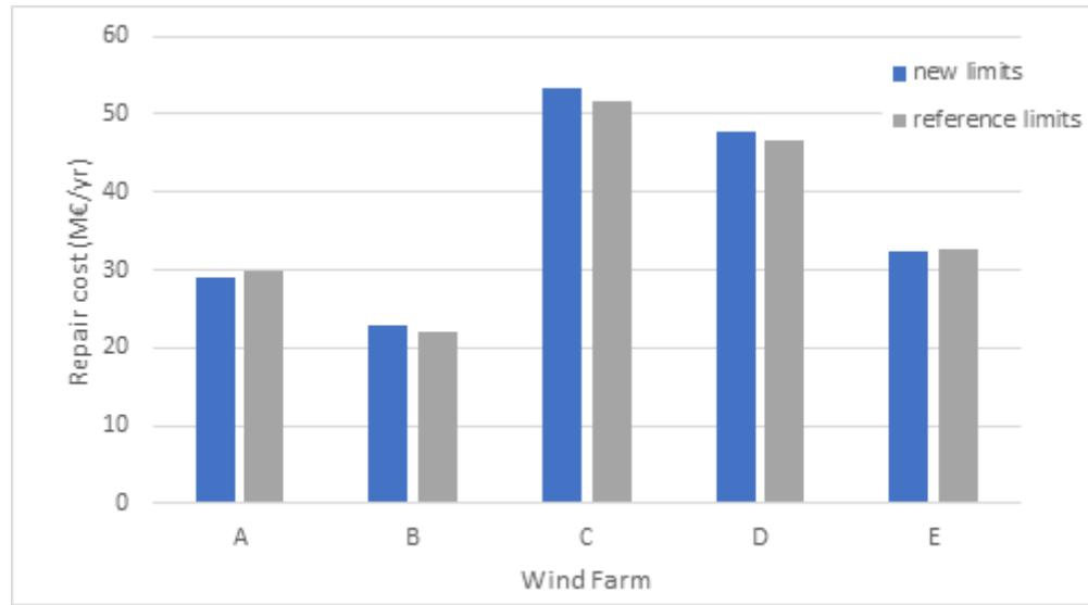
Figure 15 Comparison of repair cost for all wind farms in reference and new limits scenario
