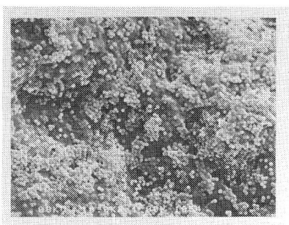
Fig.4.1a SEM photograph of a membrane of 0.12 \mu\text{m} beads without ultrasonication of the membrane mixture.
