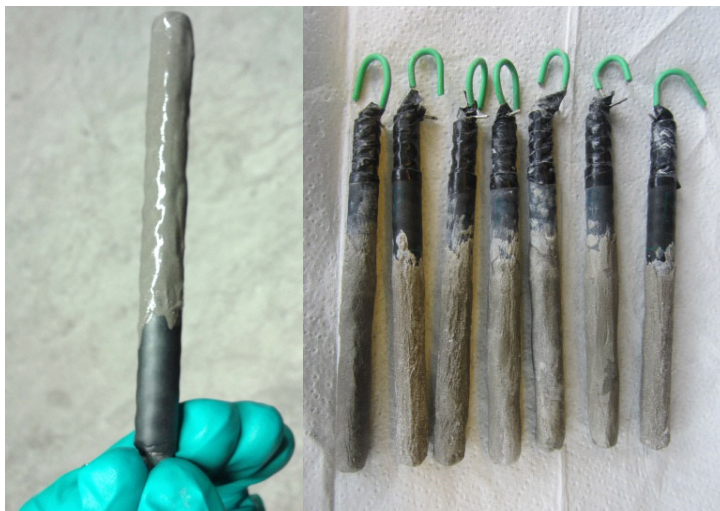
Figure 2. Freshly coated steel bars (left) and coated bars (right) after being cured for 24 hours in a fog room
