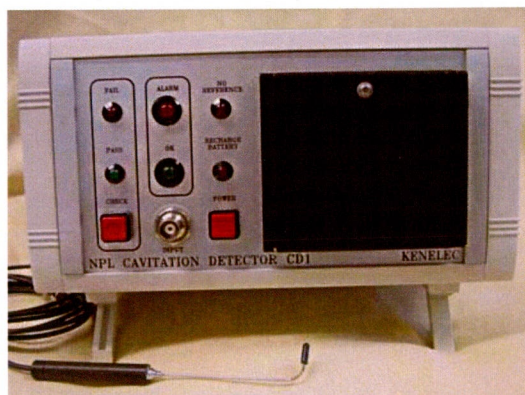
Fig. 6. The Cavitation Detector
