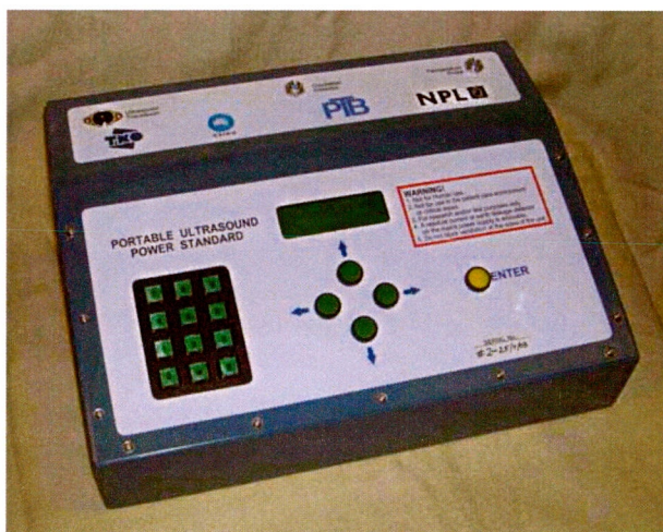
Figure 4. The Driver of the Portable Power Standard (PPS)
