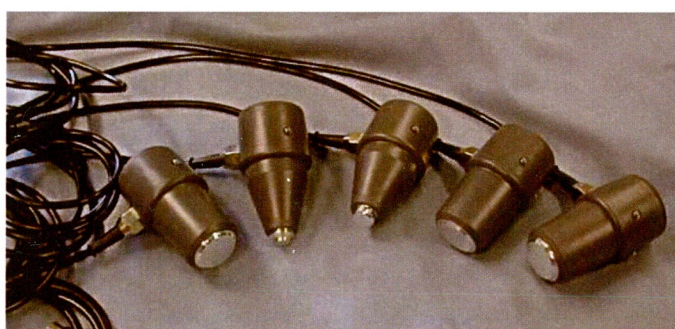
Figure 1. A finalised set of transducers to be used with the Driver of the PPS
