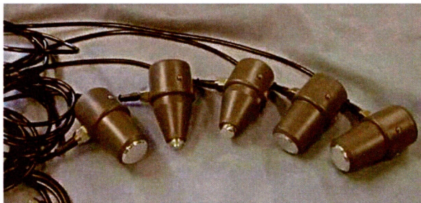
Ultrasound transducers to be used for calibration
