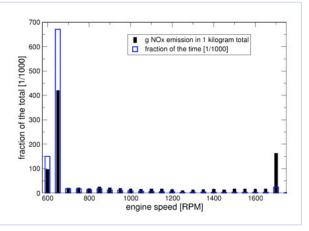
For most of the time the diesel locomotives are idling.
