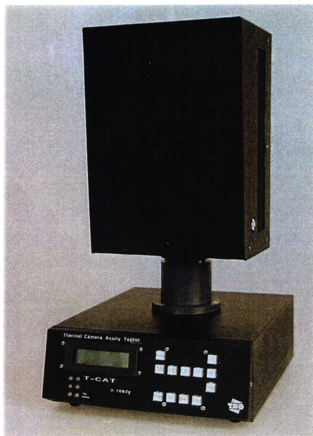
T-CAT: Thermal Camera Acuity Tester. The triangular thermal test patterns are generated in the top part. The control electronics and power supply are housed in the base.
