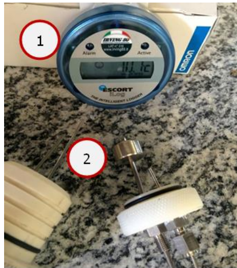
Figure 413: Reference (1) and under-test (2) thermocouples
