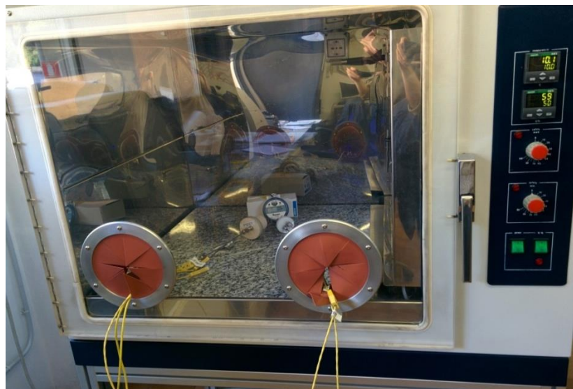
Figure 412: Temperature-controlled enclosure used for thermocouples check.
