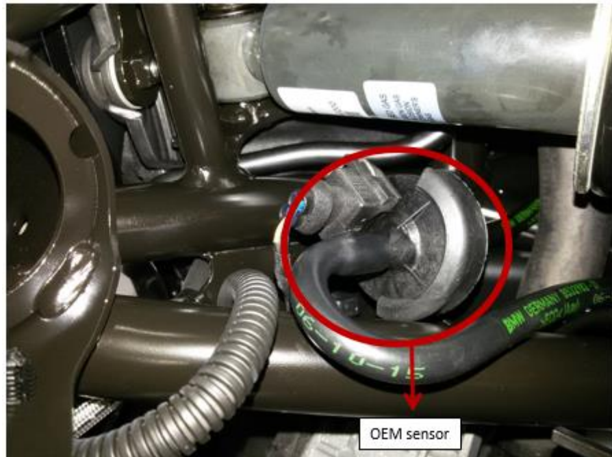
Figure 423. Sensor connections to a test vehicle measuring manifold pressure
