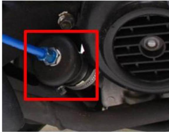
Figure 1: Connection at dip-stick hole
