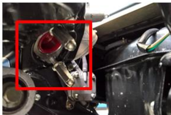
Figure 6: Exhaust opening plugged
