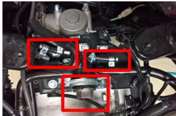
Figure 5: Intake manifold plugged
