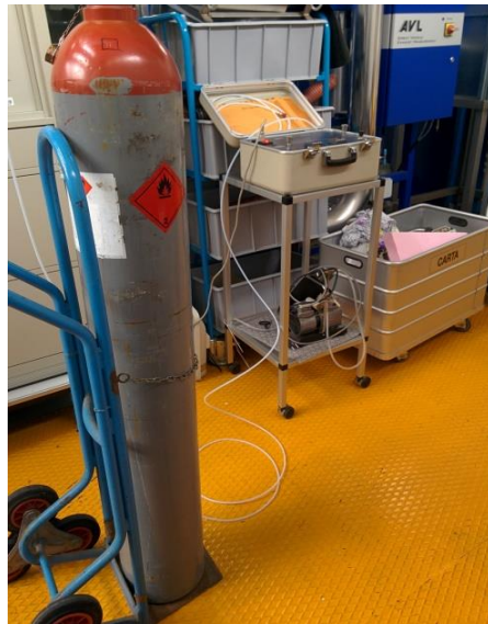
Figure 415: CFO device and propane bottle used for the retention test
