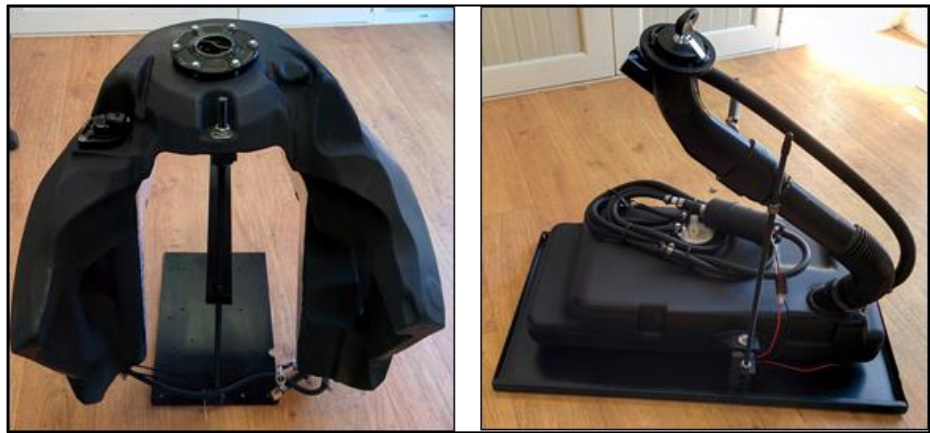
Figure 40: Fuel delivery system test rigs containing the fuel tank and fuel hoses of the vehicles.
