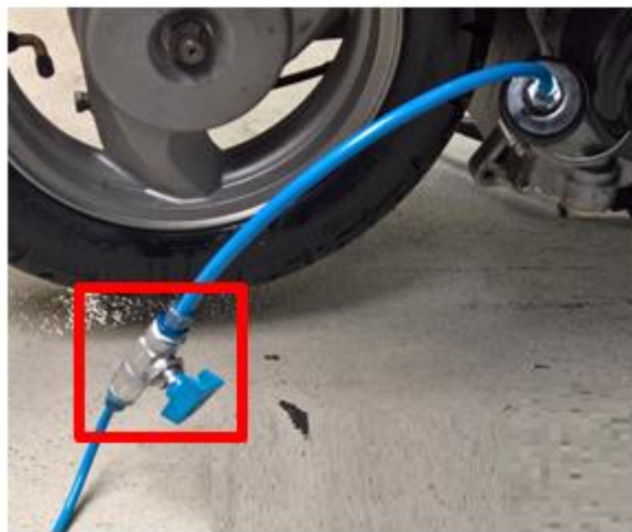
Figure 3: Connection at dip-stick hole with installed valve
