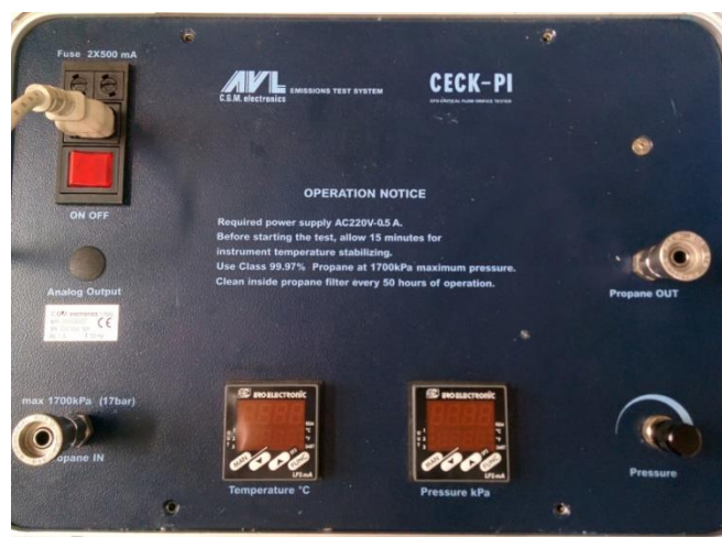
Figure 416: CFO device control panel
