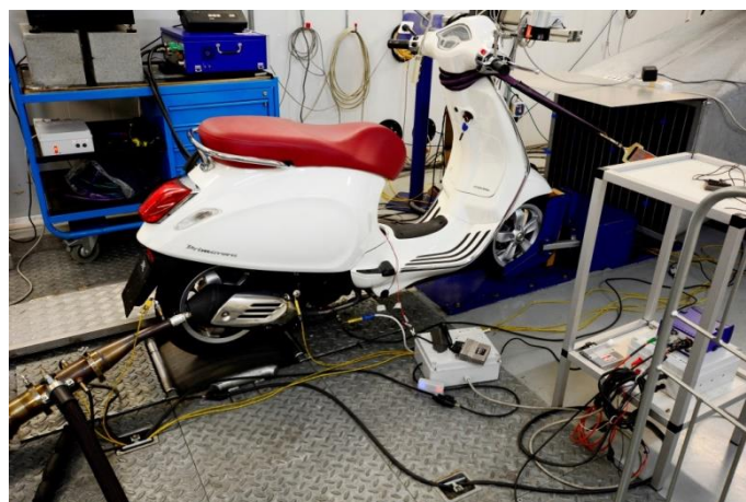
Figure 31: Vehicle on the chasis dyno during the preconditioning phase
