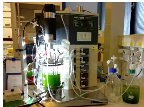
Fig. 3. Left. Graph depicting the cultivation of a Chlorella sp. culture in a CSTR: dry weight concentration in the CSTR (red squares); points at which the harvested absorption medium was reloaded with CO 2 and recycled into the system (blue diamonds). Right. 2 L-CSTR setup used for the experiments, including feed and harvesting bottles.
