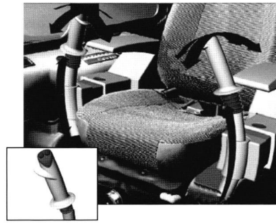
Figure 7.5 Concept 'Wheel': two traditional joysticks are coupled and can be moved as a steering wheel. This creates extra steering functions with a good support
