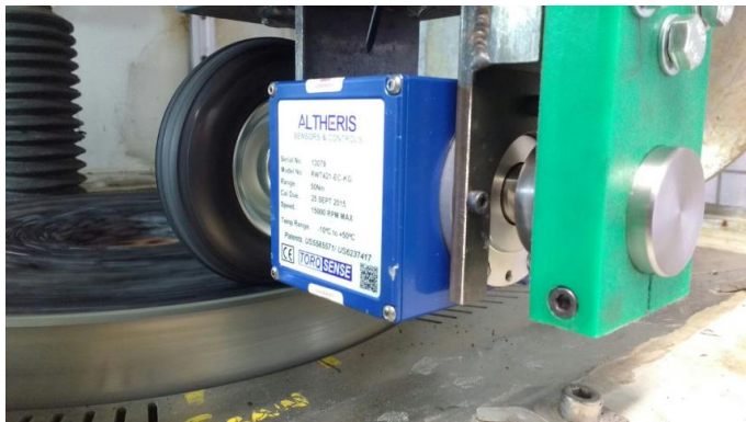
Figure 2: Measuring rolling resistance on an asphalt
