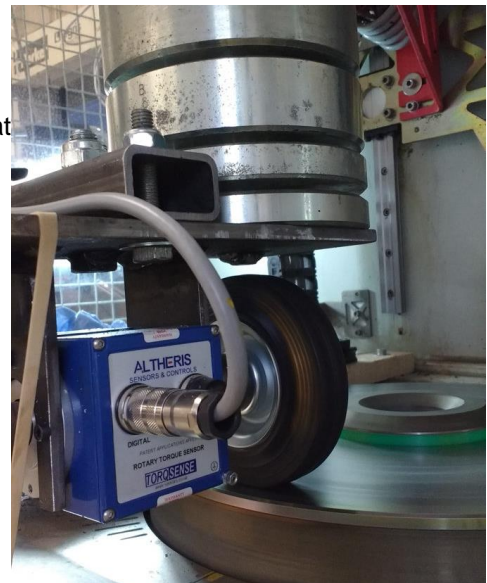
Figure 3: Measuring rolling resistance on a steel plate
