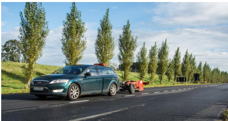
Figure 1: Rolling resistance measurement on the test section in
