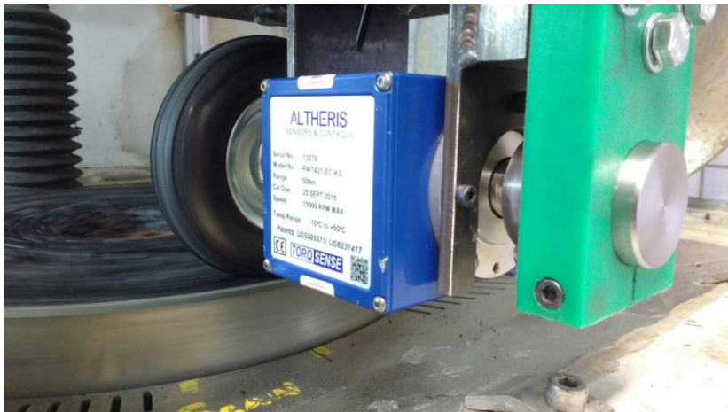
Figure 2: Rolling resistance on an asphalt layer in the laboratory
