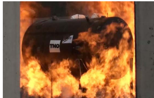
Fig. 2. Double walled tank containing cryogenic liquid engulfed in fire during the experiment
