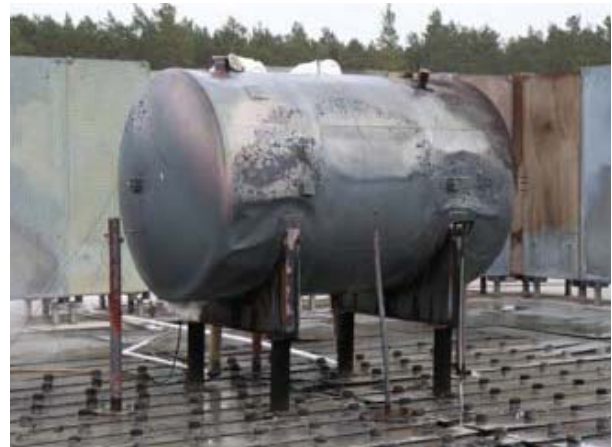
Fig. 5. Cryogenic tank after the fire test
