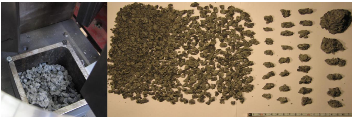
Figure 4.32 Photographs of the post-failure fragments of a porous concrete (PRC1)
