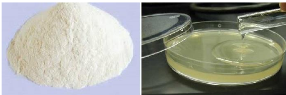
Figure 2.2 Agar as additive to increase surface tension (Fankhauser 2010)
