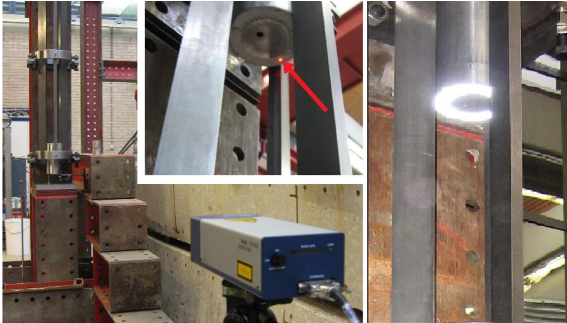
Figure 4.15 Test set-up, laser vibrometer sensor head and the bottom surface of the impactor
