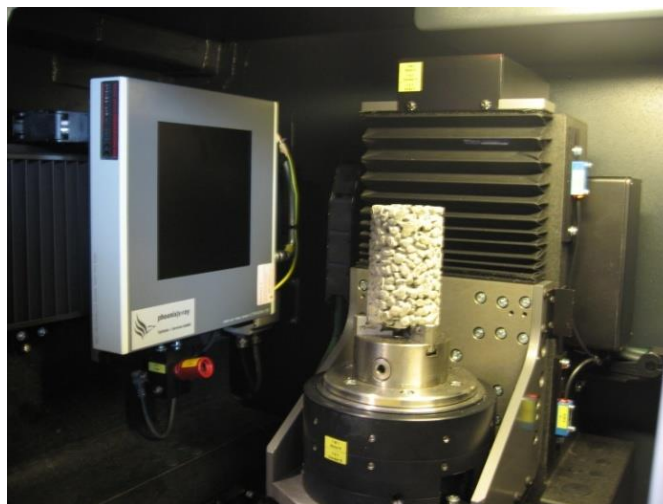
Figure 3.6 Computed Tomography (CT) machine for testing building materials
