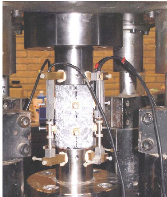
Figure 3.1 Deformation controlled uni-axial compression test set-up
