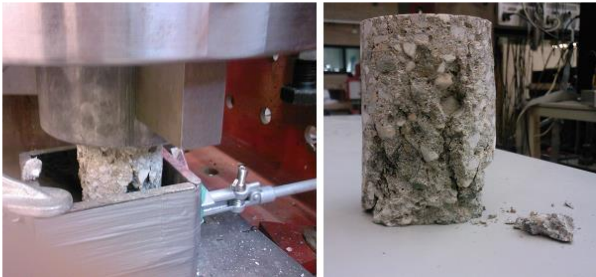
Figure 4.33 Photographs of the post-failure fragments of a normal concrete (NC1)
