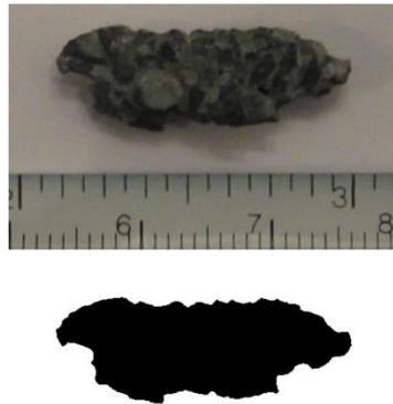
Figure 4.34 Post-failure fragment and its maximum projected profile
