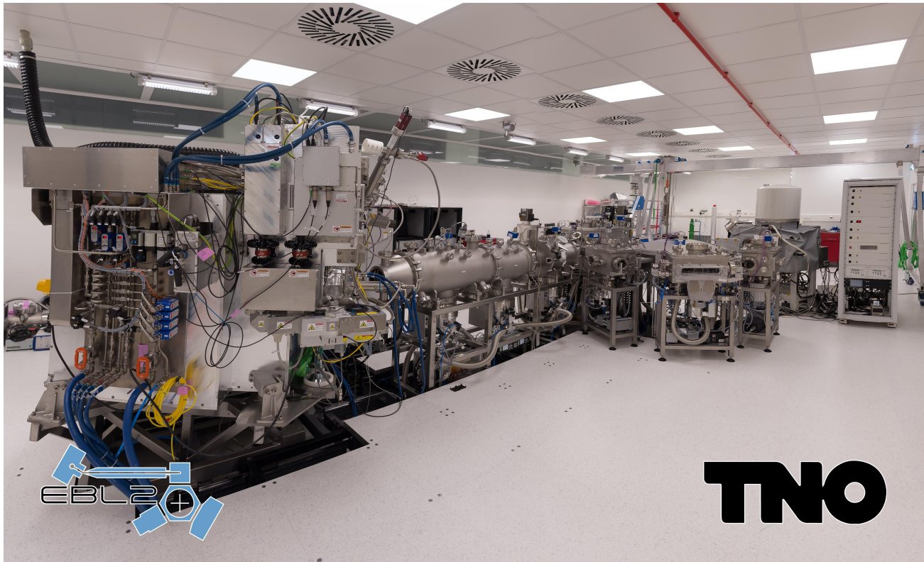
Figure 4: Full view of EBL2, from left to right: EUV source, collector module, exposure chamber, vacuum handler with load lock, storage, and XPS. The atmospheric handler with pod opener is not yet present.
