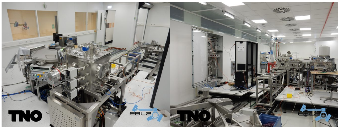
Figure 3: EBL2 in stages of assembly. On the left side the exposure chamber and vacuum handler. On the right side the XPS is arrived on site (right side of photo), in the front the source frame is visible and the rails for moving source and collector module.
