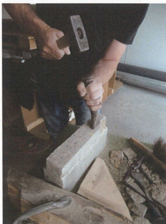
Fig. 4. Making of a mullion by hand.
