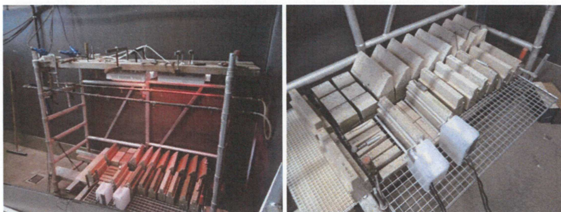
Fig. 6. Overview of weathering test (left) and specimens used for the test (right).
