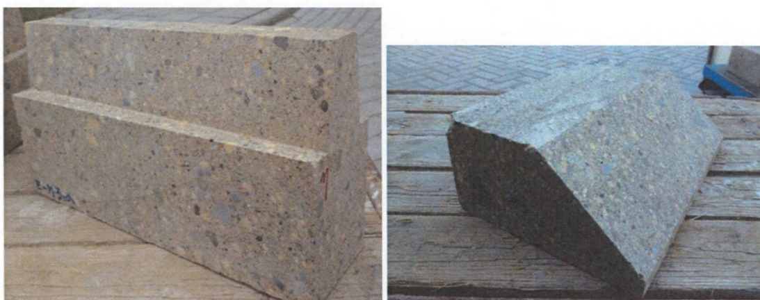
Fig. 3. Examples of cut mullion and window sill.
