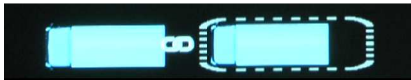
Figure 2.2 Screen shot of the interface showing the lead truck (left) and following truck (right) with the activation zone (dashed square) when the automation was switched on the colour changed from white to blue and the linking symbol was displayed between the two trucks.
