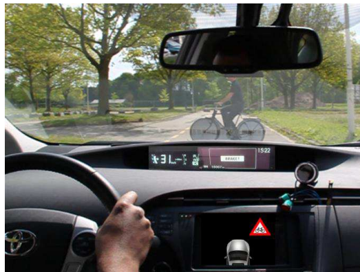
Fig. 2. Toyota Prius with C-AEB warnings.
