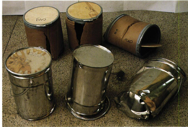
Resulting damage of solid and liquid packagings after 12 m droptest.
