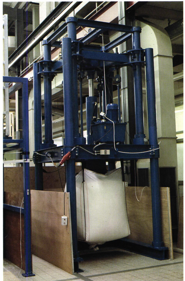
Top lift testing equipment for flexible IBC's.
