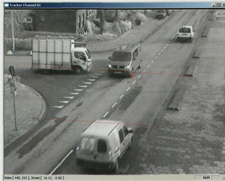
Figuur 6 - Location 1: Pijnacker as seen from one of the two video cameras with the reference points for the transformation from the image plane to the plane of the street in blue and an example of a vehicle measuring point in red.
