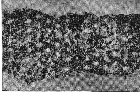
Figure 28 Example of the bonding surface of a cross section of a sm-RIJ specimen after failure (the dark area in the middle corresponds with the actual bonding area)
