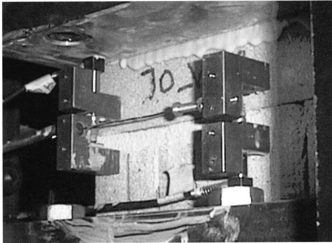
a) brass brackets with LVDT's on specimen
