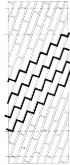
Figure 81 Example of four potential oblique cracks, anticipated in a JO.70 specimens
