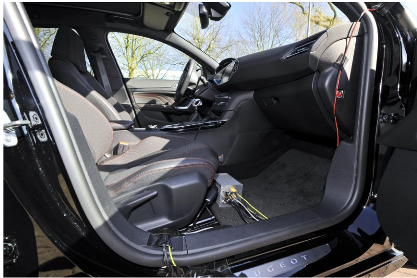
Figure 15: The SEMS system, developed by TNO, mounted on a vehicle to be tested on the road.
